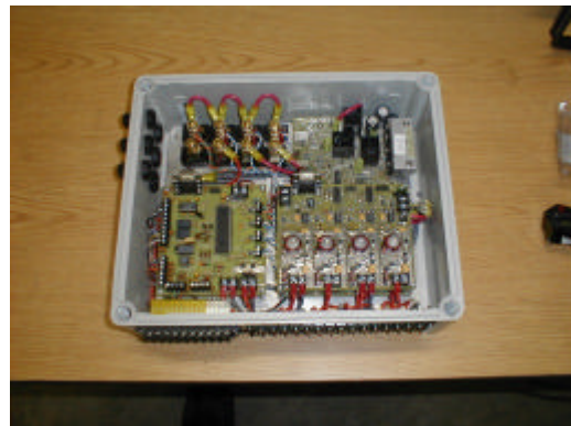
Figure 2. Microship Power Control System
